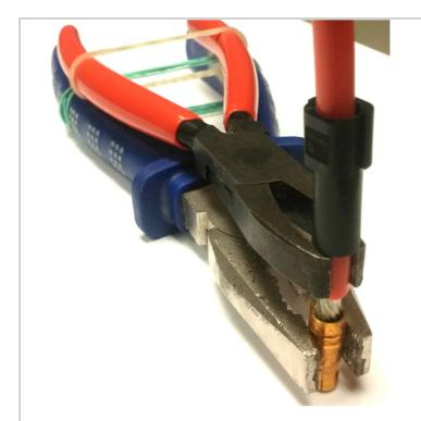
Wrap rubber bands around both plier's handles. Build a stack as shown above and clamp the contact element in the lower one, and the cable in the upper one. Carefully insert all strands of the cable core. Make sure not to forget the contact housing in this setup! I know what I'm talking about...
