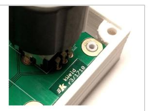
Push the circuit board into the lower shell. Ensure the correct orientation by matching the foot switch cable with the corresponding cutout. Make sure that all four edges are completely sunken into position as shown on the right.
