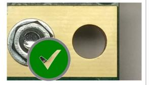
Make sure that the two 6mm holes are correctly aligned before fastening the screws.
