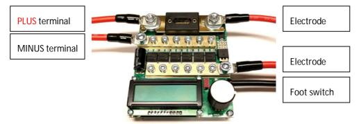
To complete the kit and make it operational, you need to connect it to a suitable power source. The *kWeld* operation manual discusses its requirements and a number of different options; this is not within the scope of this document.
