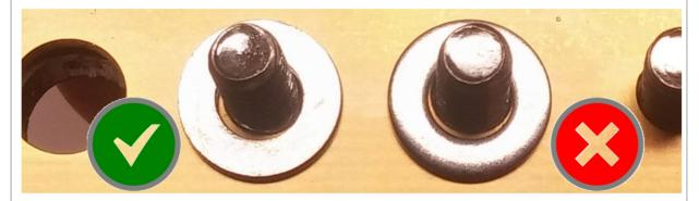
Observe correct orientation of the washers, you may damage the circuit board otherwise.
