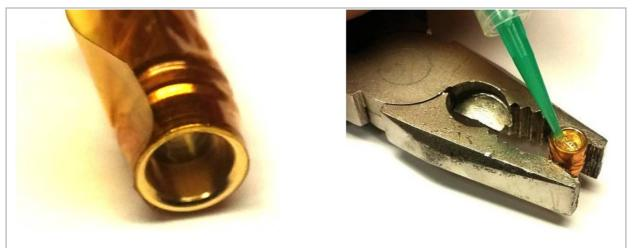
Wrap a few lsyers of Kapton tape around the XT150 contact element (left picture). This serves two purposes: it adds thermal insulation and eases soldering when the element is clamped in the pliers, and it prevents solder from flowing down the sides of the element. Pour some tack flux into the cup as shown in the right picture. Fill roughly 1/5 of the cup depth.
