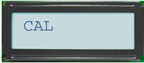
Shown when the system has not been calibrated yet. **NOTE:** because the system is shipped in this condition, this is the first screen that you will see. You need to perform a calibration once before the welder can be used. See section "Calibration" on page 15 for details.
