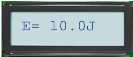
The displayed value is the commanded energy in Joules that shall be dumped into the weld spot with the next trigger. Use the dial knob to adjust this to a level that is suitable for your weld material. The following table gives some values for different materials when used in combination with 18650 type cells. Use them as a starting point only and experiment to find the best adjustment for you, before beginning productive work.
