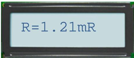
*The calculated average resistance of the weld spot (in milliohms).*
