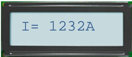
*The average current (Amperes) that was flowing through the weld spot.*
