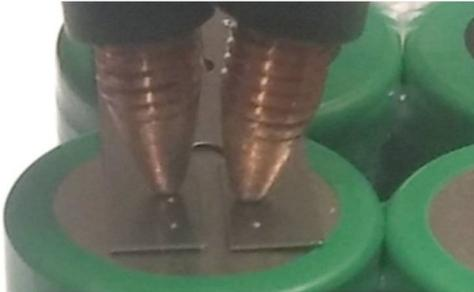
2. Trigger a pulse by stepping on the foot switch - and keeping your foot down. Don't be frightened, the cables will jump from the high current flowing through them, and the weld spot may emit sparks. You'll see the LCD illumination dim briefly - this is done on purpose to save power during the pulse.
