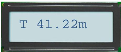
*The pulse duration (in milliseconds) that was necessary to achieve the requested energy level.*
