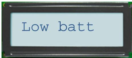
You have enabled a battery voltage warning level, and the battery voltage is lower than that.
