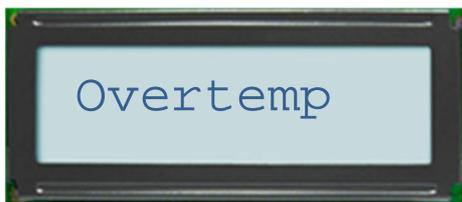
The power switch temperature is above 70°C and needs to cool down before continuing.
