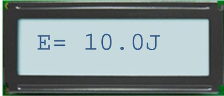
Ready to weld! The screen shows the energy in Joules that will be used for the next weld. Turn the dial knob to adjust this value. Continue reading the next sections to learn how to make welds in manual or automatic mode.
