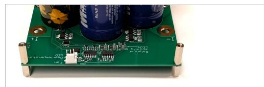
Mount the four 15mm standoffs from the housing kit to the top side of the module as shown, using the existing 10mm standoffs from the *kCap* kit.
