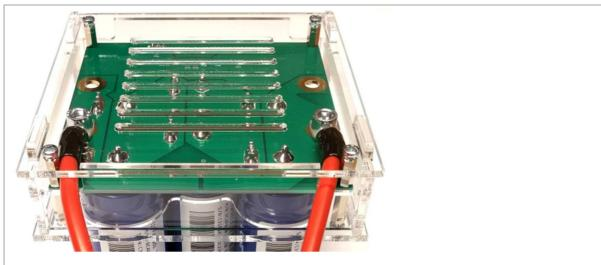
Attach the bottom cover (this part is also symmetrical) using the remaining four M3 screws. Again, fasten the screws gently.
