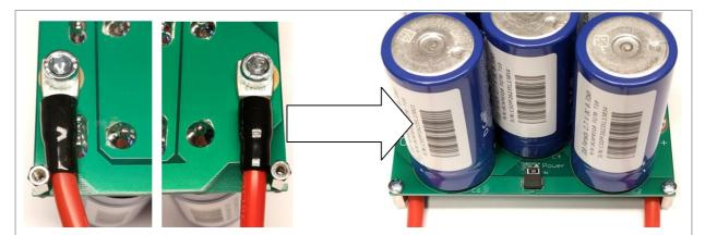
Use the M6 screws, washers and nuts to attach the cable assemblies to the module's underside. Tighten the nuts with securely. Observe correct orientation of the washers, you may damage the circuit board otherwise. Use the stacking scheme as shown below on the right.
