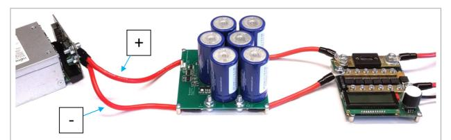
Connect the cables to the input terminals of the *kCap* module as shown.
