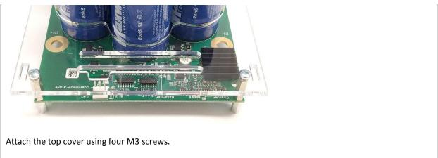
NOTE: fasten the screws gently; acrylic glass may crack when applying too much torque.
