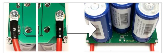
Use the M6 screws, washers and nuts to attach the cable assemblies to the module's underside. Tighten the nuts with securely. Observe correct orientation of the washers, you may damage the circuit board otherwise. Use the stacking scheme as shown below on the right.
