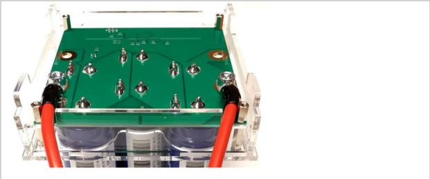
Flip the module upside down, and slide the four side wall parts into place as shown above. The parts are symmetrical.
