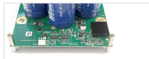
Mount the four 15mm standoffs from the housing kit to the top side of the module as shown, using the existing 10mm standoffs from the *kCap* kit.
